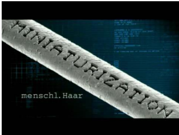
Fig: A laser was used to write into a human hair.
